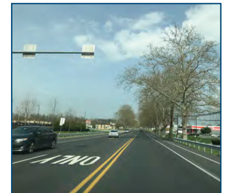
Figure 5.5: The existing bike lane east of Continental Way ( Map D ) is adjacent a wide travel lane with a posted speed limit of 45 mph. It is recommended that design changes be implemented along this segment to produce a consistent operating speed of 30 mph. Potential design changes include reducing the width of the travel lanes.
